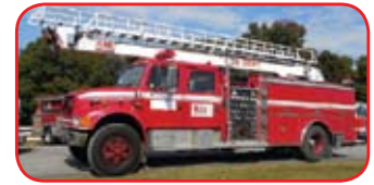
1992 3D Int'l 55' Firestix International 250 HP Diesel Hale 1250 GPM Pump 500 Gallon Steel Tank
